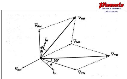
From phasor diagram, it is clear that phase angle between  $V_{YB}$  and  $I_Y$  is (30° +  $\varphi$ )
